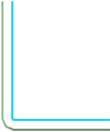
15, 'quad_segs=4 join=bevel' shown with original line
