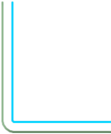
15, 'quad_segs=4 join=round' original line and its offset 15 units.
