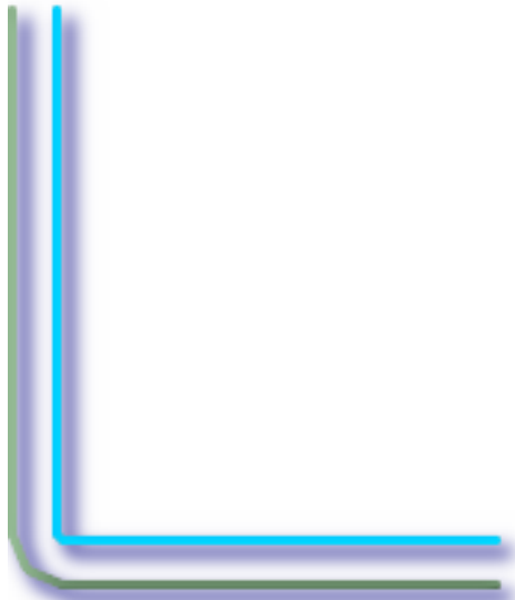
15, 'quad_segs=4 join=bevel' shown with original line
