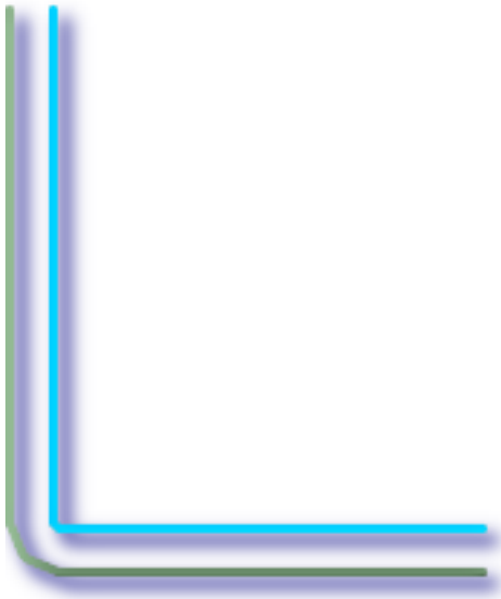
15, 'quad_segs=4 join=bevel' shown with original line
