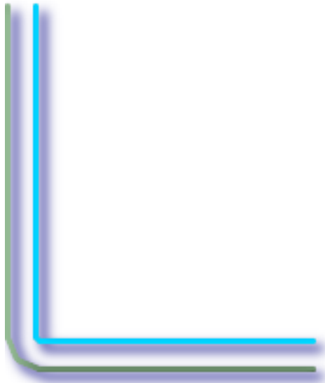
15, 'quad_segs=4 join=bevel' shown with original line
