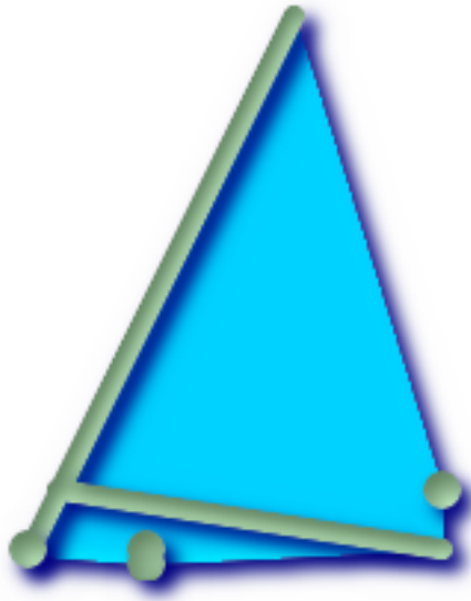
Convex Hull of a MultiLineString and a MultiPoint seen together with the MultiLineString and MultiPoint
