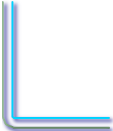
15, 'quad_segs=4 join=bevel' shown with original line
