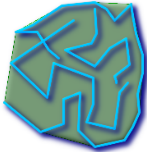
multilinestring overlaid with Convex hull
