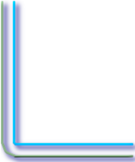
15, 'quad_segs=4 join=bevel' shown with original line
